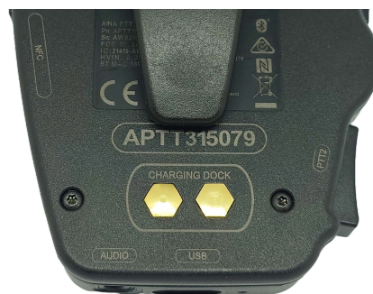
Figure 3: Friendly name printed at the back of the PTT Voice Responder (example image)
