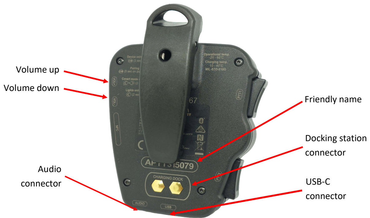
Figure 2: Rear view and connectors
