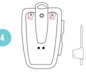
Insert the battery back into the device so that the battery contacts align and the battery label faces into the device. Then slide the battery cover back into place and screw it shut. Do not over tighten.
