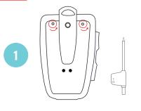
Turn off the device. Open the battery cover with the provided screwdriver and remove the device's battery.
