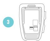
Make sure the inside of the device is clear of any dust and dirt, specially the grey area shown, to ensure the watertightness of the device.
